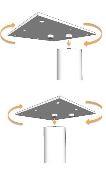
\*The mounting plate must be securely fastened to the post for a trouble free installation. There can be **NO GAP** between the post and the mounting plate.
